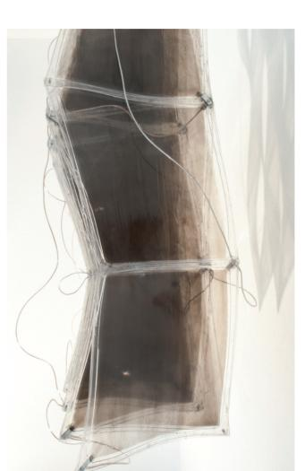
EAP is a polymer actuator that converts electrical power into mechanical force. In principle it consists of a thin layer of very elastic acrylic tape sandwiched between two electrodes. Once the voltage in the range of several kilovolts is applied between the electrodes, the polymer changes its shape in two ways.
